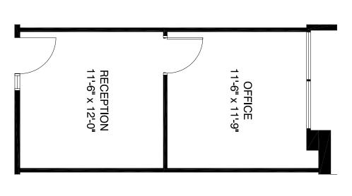
CALCULATION LINES HAVE BEEN TAKEN TO TENANT SIDE OF PUBLIC CORRIDOR, TENANT SIDE OF CORE WALLS, AND INSIDE SURFACE OF DOMINANT PORTION OF EXTERIOR WALL. RENTABLE FACTOR IS 1.1312 AS PREVIOUSLY ESTABLISHED BY OTHERS. idGROUP HAS NOT BEEN AUTHORIZED TO CONFIRM CODE COMPLIANCE.
